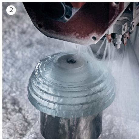
Grinding and polishing on CNC machine.
